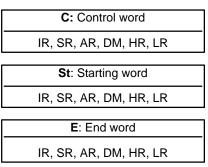
St and E must be in the same data area, and St must be less than or equal to E.
